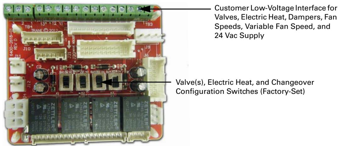
**Figure 6. CSTI adapter board field connections**
