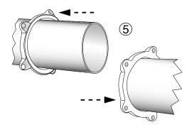
**Step 6** • Lubricate the gaskets and pipe surface with a suitable gasket lubricant.
